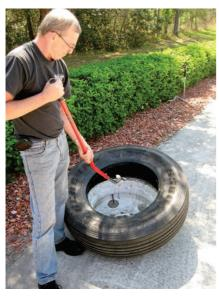
1. Position the wheel drop center down and position a clean, properly lubricated tire for mounting.
