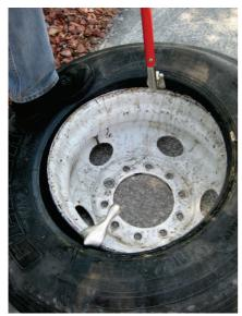
3. Place bead keeper on the wheel to hold the bead as the tire is mounted. Begin working around the edge where the bead is not yet mounted.
