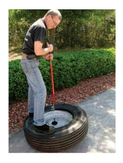
3. Stand on the tire to retain the bead. Begin working at one edge where the bead is not yet mounted.
