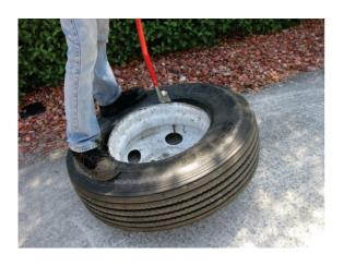
4. Use the Golden Buddy Mount bar to pry the bead onto the wheel. Continue working the wheel until the tire is mounted. It may be necessary to widen your stance.
