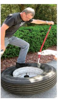
4. Use the Golden Buddy mount bar to pry the bead onto the wheel. Continue working around the wheel until the tire is mounted.
