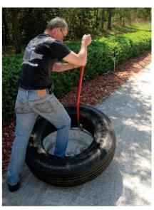
2. The Golden Buddy mount bar maybe used to press the first bead over the lip allowing the bead to fall into the rim gutter.
